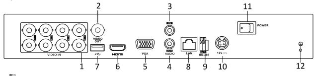
**NOTE** The rear panel of AR314-4 and AR314-16 provide 4 and 16 video input interfaces respectively.
